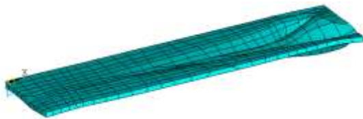
Figure 9. Geometry of wing profile – as imported from IGES file
