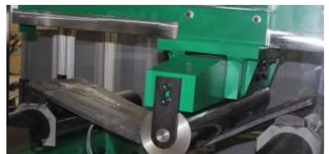
Figure 8. Deflected wing profile during experiment
