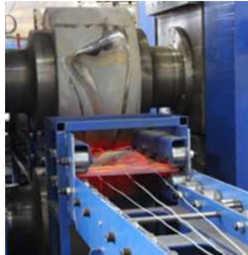
Figure 1. Production of hot rolled wing profile.
