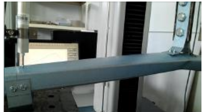
Figure 6. Deformation of the wall plate system
