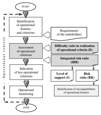
Figure 1. Scheme of the operational control in consideration of the assessment of operational criterions.
