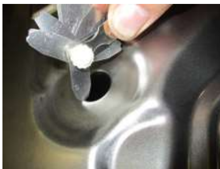
Figure 9. (c) Flanged hole validated using numerical simulation with the support of AutoFORM software- Experience number 8.
