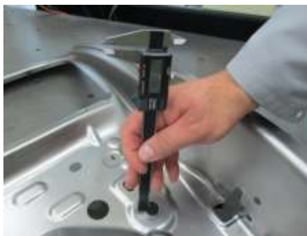
Figure 9. (b) Flanged hole validated using numerical simulation with the support of AutoFORM software- Experience number 8.
