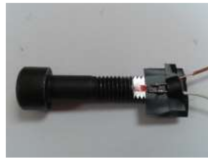
Figure 7. Strain gauge located at the stem
