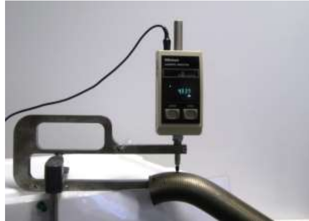
Figure 3: The wall thickness measuring device
