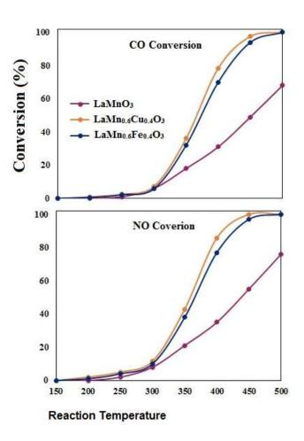
Fig. 3: Temperature profile for NO and CO conversion over LaMn0.6B0.4O3
