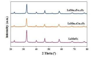
Fig. 1: XRD patterns of LaMn<sub>0.6</sub>B<sub>0.4</sub>O<sub>3</sub> samples
