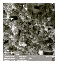
Figure 6. Microstructure of geopolymer (50 wt % red mud, volcanic tuff "Strmoš", 8 wt % metakaolin, magn. 5800 X)
