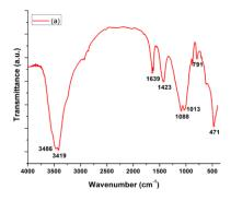
Figure 5. FTIR analysis of geopolymer (50 wt % red mud, volcanic tuff "Strmoš", 8 wt % metakaolin)
