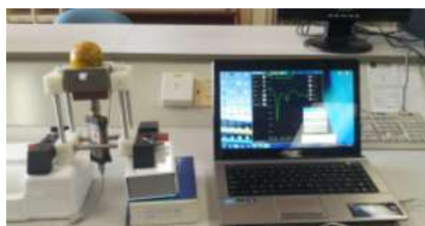
Figure 2. (a) Nylon holder filled with oranges sample (b) Measurement of reflection coefficient using monopole sensor and CABAN R54 Reflectometer
