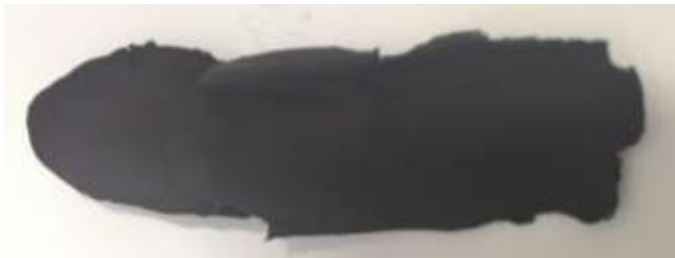
Figure-4. Stabilized PAN nanofiber webs which were subjected to carbonization and activation
