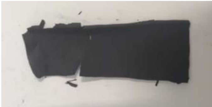
Figure-3. Stabilized PAN based carbon nanofiber which was carbonized in nitrogen gas for 45 min.
