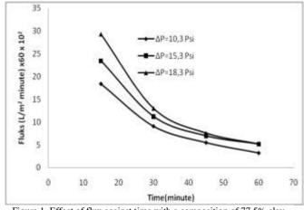
Figure 1. Effect of flux against time with a composition of 77.5% clay, 20% rice bran, 2.5% iron powder with rice bran size of 500 μm and an iron powder of 250μm.
