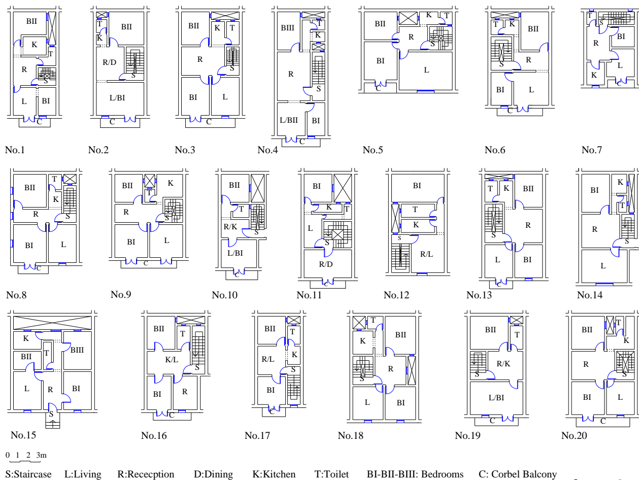
Figure 7. Typical Floor Plans of Survey Buildings in 2015
