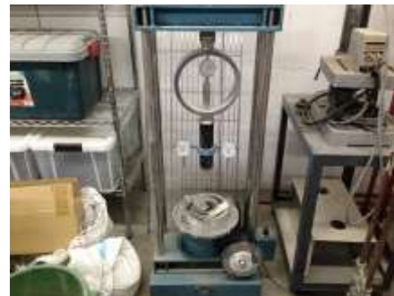
Figure 4 Penetration device used in CBR test
