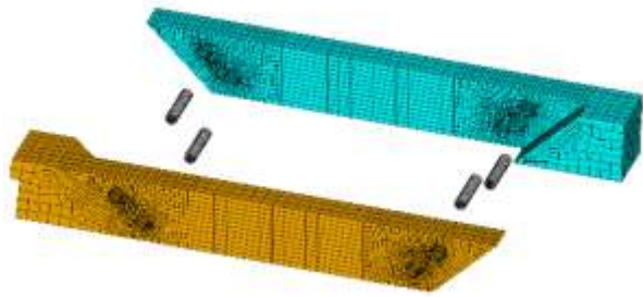
Figure 5. Numerical model of four-dowel joint in ANSYS software
