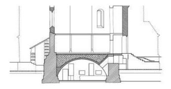
Figure 1. Cross section of a medieval stone church in Wroclaw (Poland), different shape and contour of the foundation in relation to the main body of the church is visible.
