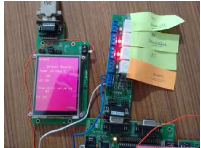
Figure 5: Operation of actuators AC & dehumidifier
