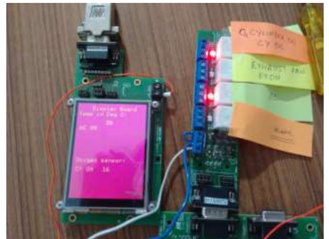
Figure 6. Operation of actuators AC & oxygen cylinder
