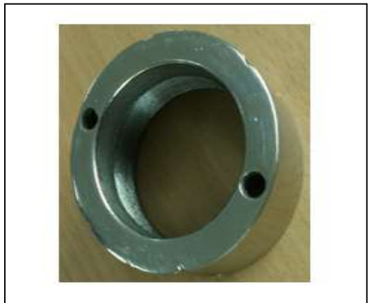
Fig.2: Clamp Sleeve which is located inside the crimping head and outside the inside the crimping head and outside the crimping tong
