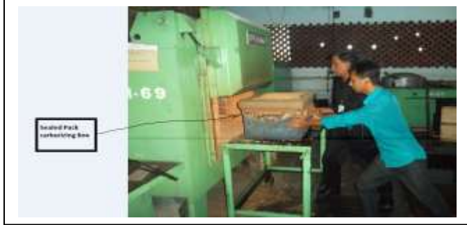
Fig. 6: Pack carburizing Box inserted to the Furnace
