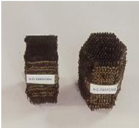
Fig: 7 3D, 4D woven preforms
