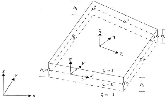
Figure 2 Coordinate system for 8-noded degenerated shell element
