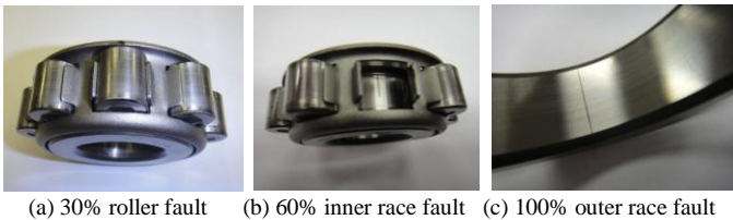
Figure 6. Photo of fault bearing
