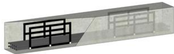
Figure 1. Schematic view of concrete beam reinforced with GFRP plates proposed in this study
