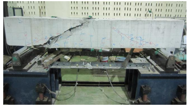
Figure 5. Shear compression failure
