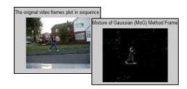
Fig.4 Background Subtraction using Mixture of Gaussian
