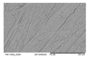
Figure 4: SEM image for carbon steel 1 after 3 h of immersion in  $1M\ HCl + 1g/L\ A$ . Herba Alba.
