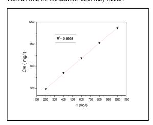
Figure 2: Langmuir adsorption plot for carbon steel in 1M HCl containing different concentrations of A.herba alba.
