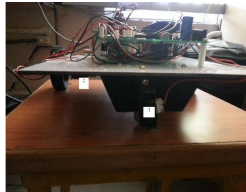
Fig 7. Obstacle sensor fixed in the embedded vehicle 1. Obstacle Sensor 2.Stepper Motor
