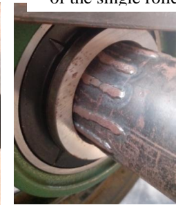
Fig. 4—welds to account for difference in diameter
