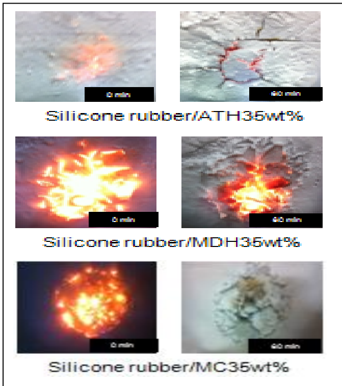
Fig. 5 Tests of fire resistance for each flame retardant (Left; Start, Right: End)
