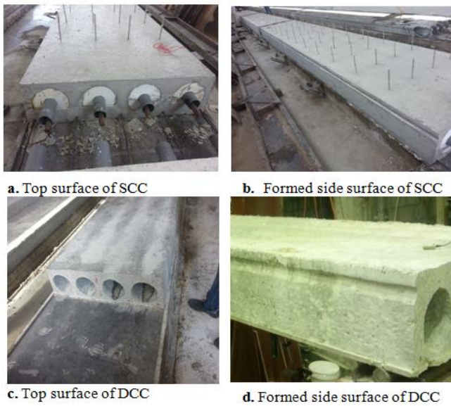
Figure 6. Surfaces of SCC compared with DCC.
