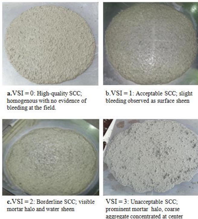
Figure 5. Development of SCC slump flow (ASTM C1611).
