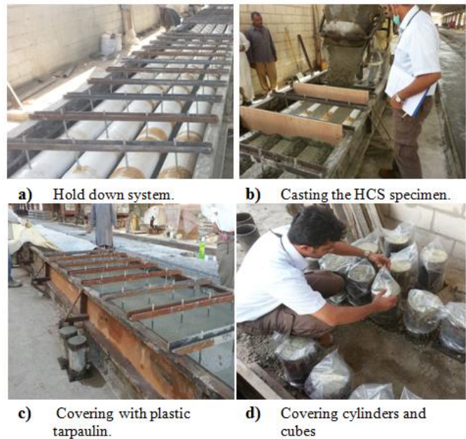
Figure 3. Preparation and casting procedure.
