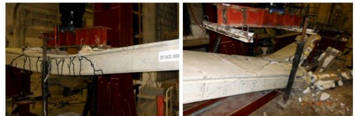
b. Flexure failure mode for HCS specimen ST-SCC-300.
