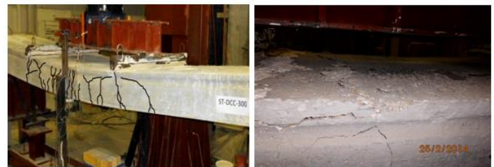
a. Flexure failure mode for HCS specimen ST-DCC-300.
