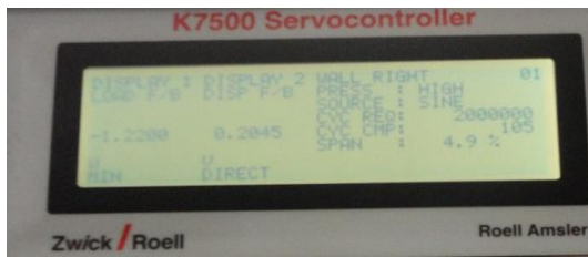
Fig. 1b: Dynamic loading sine wave input shown on K7500 Servocontroller for -1.2200V
