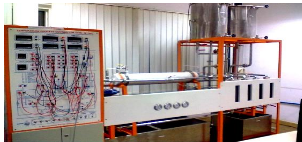
Fig.1. Heat Exchanger Physical experimentation experimental setup
