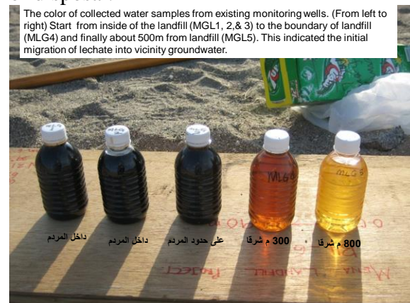
Figure 3: Groundwater samples taken from wells at different distances in the Landfill (From left to right: samples from inside landfill (2), sample from landfill boundary, sample from 300 m East of the landfill, sample from 800 m East of landfill).
