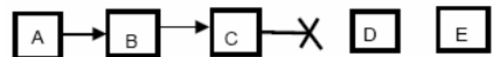
Fig.2 Node C is unable to forward a packet from A to E over the next node D
