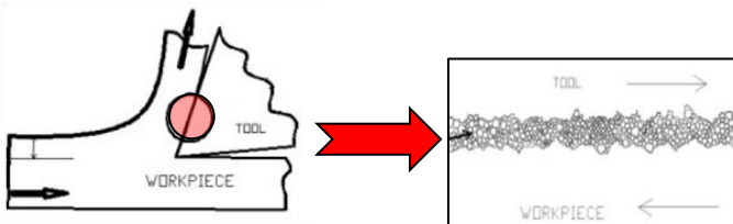
Figure 12. Rolling elements in the tool-chip interface [16]
