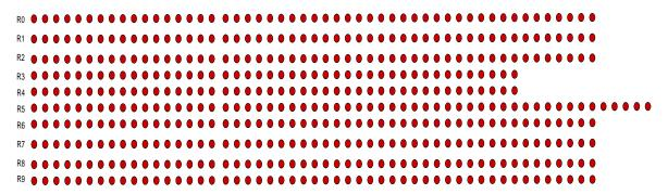
Fig. 7. The number of chip ID generation circuits on each row: R0-51, R1-51, R2-51, R3-44, R4-44, R5-56, R6-51, R7-51, R8-51, R9-51, R10-51
