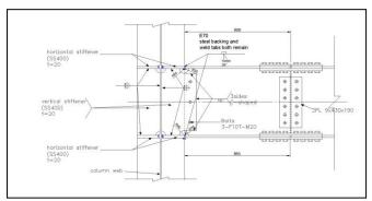
Figure 2. Detail of weak axis basic column-tree type.
