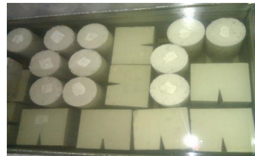
Figure 3. Experimental samples are in the cure.
