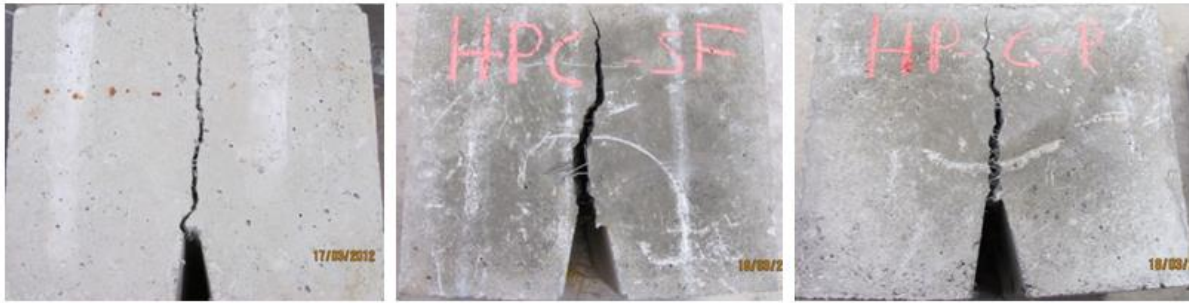
Figure 6. Fracture types of normal and high strength concrete with fiber.
