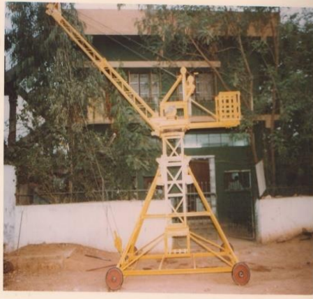
FIG.03 : WHEELED UNDER CARRIAGE FOR MOBILITY OF MINI CLIMBING CRANE AT SITE.
