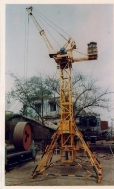
FIG.01 : MINI CLIMBING CRANE AT WORK IN A YARD
