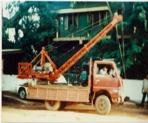
FIG.04 : MINI CLIMBING CRANE MOUNTED ON TRUCK CHASSIS FOR TAXI SERVICE IN MATERIAL HANDLING AT DIFFERENT NEARBY SITES.
