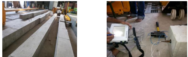
Figure1. Experimentally tested specimen and Pulse Echo configuration Instrumentation
