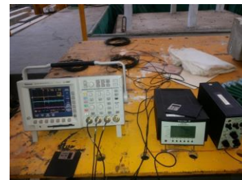
Figure3. Instrumentation for Pitch catch configuration method
