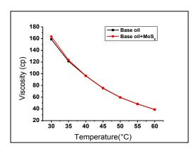
Figure 8. Variation of viscosity with temperature.
