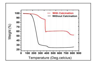
Figure 5. TGA thermograph of MoS<sub>2</sub> nanoparticles.
