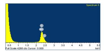
Figure 4. EDX pattern of MoS<sub>2</sub> nanoparticles.
