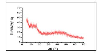
Figure 3. XRD pattern of MoS2 nanoparticles.
