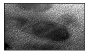
Figure 1. Lamellar structure of MoS<sub>2</sub> nanoparticles.
