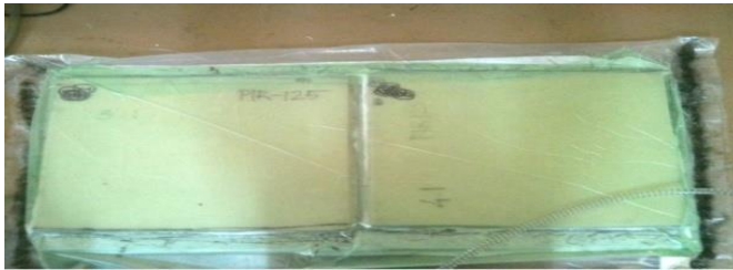
Figure 2: Vacuum bagging process
