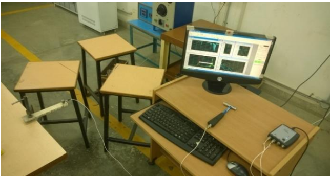
Figure 4: Impulse hammer experimental setup
