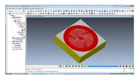
Fig. 4 Roughing view of the Cavity
