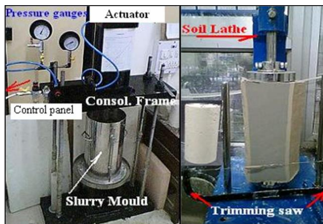
Fig. 2. Consolidation setup on the laboratory floor
