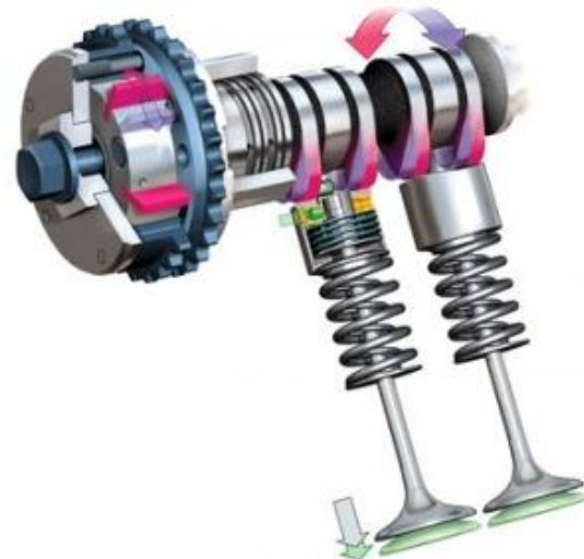
CAM operation according to variable valve timing
