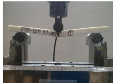
Figure 3. Three-Point bending testing of 125kg/m<sup>3</sup> 12:1 specimen on Instron machine
