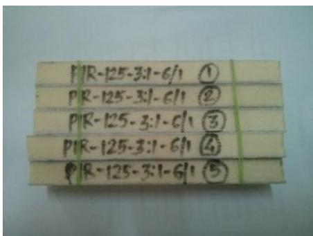
Figure 2. PIR 125kg/m<sup>3</sup> weight ratio 3:1 and span to depth ratio 6:1 specimens
