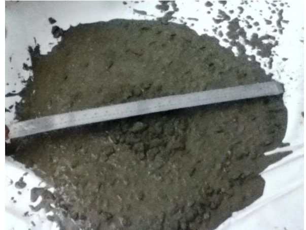
Fig.1: Slump test (Flow ability)
