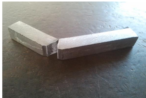
Figure 5. Izod Impact testing Specimen after conducting test
