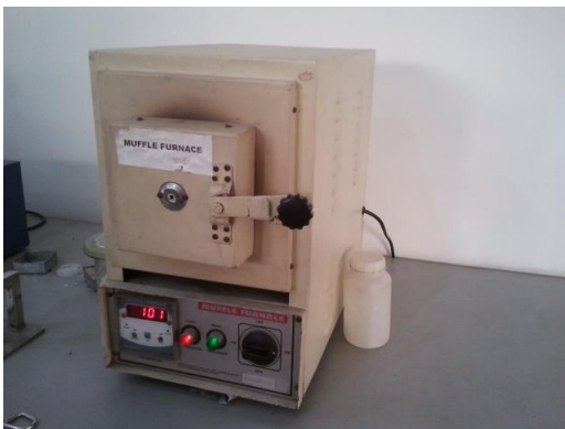
Figure 1. Rectangular Muffle furnace for heat treatment
