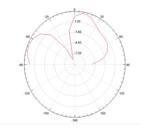
Figure 3(b) Radiation Pattern at Frequency 2.8 GHz, phi=60°
