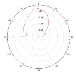
Figure 3(a) Radiation Pattern at Frequency 8 GHz, phi=60°
