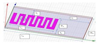
Figure 1(a) Dimensions of the Meandered Planar Inverted F Antenna
