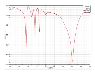
Figure 2 Simulated Magnitude of the  $S_{11}\mbox{ Parameters}$  of Proposed Antenna
