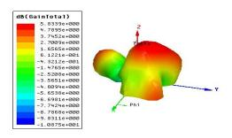
Figure 4 Three Dimensional Polar Plot of Gain
