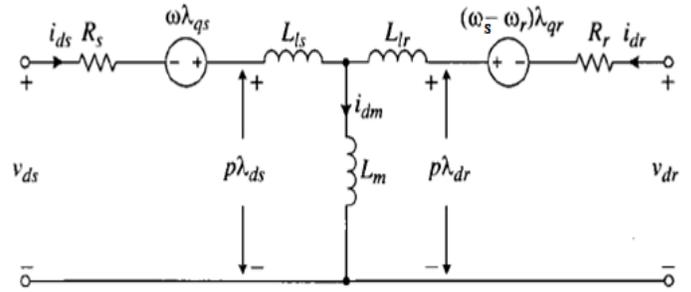
Fig.2 Equivalent circuit of DFIG in q-d axis
