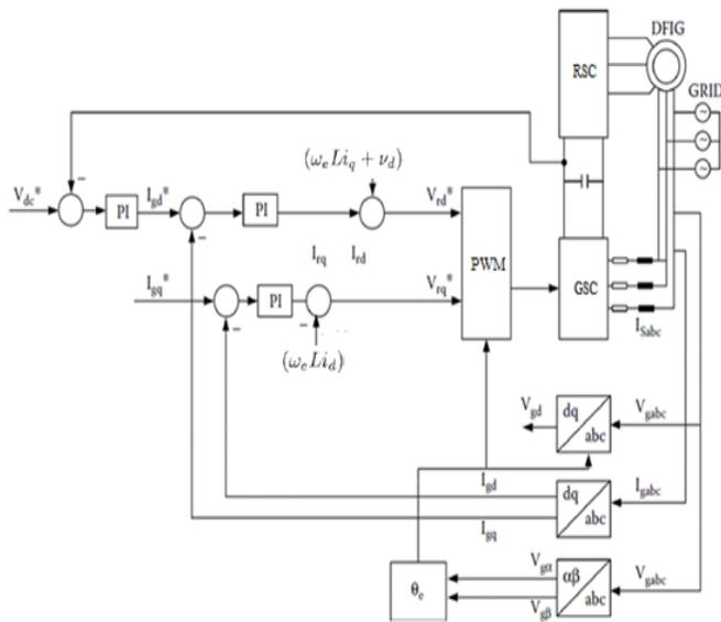
Fig 5. Schematic block diagram of GSC control.
