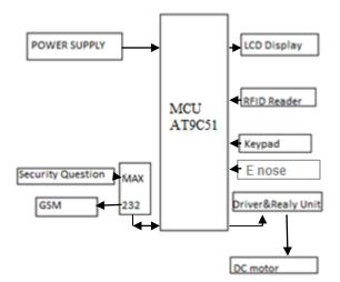
Figure 3. Block Diagram of Locker Security System
