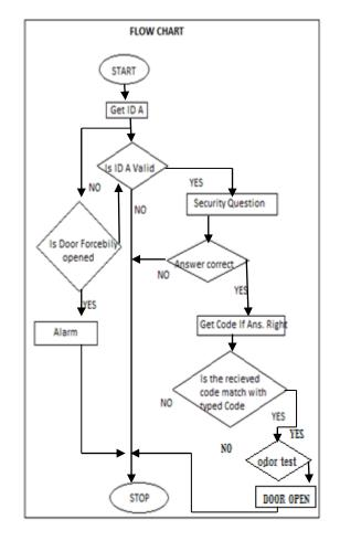
Figure 2. Locker Security System Based On RFID,GSM, Security Questions & Odor Identification
