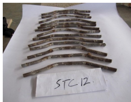
Figure 8 The hinge plastic of bolt
