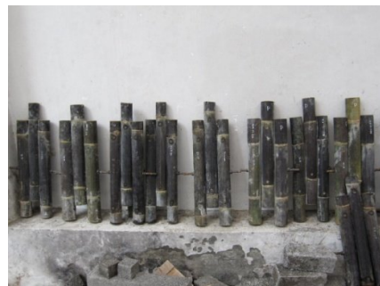
Figure 7 Specimens of three-component bamboo
