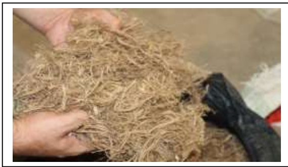
Figure 1 Kenaf fiber (cut 30mm length)
