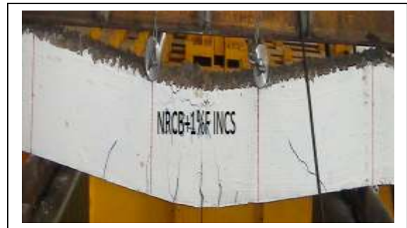
Figure 11 RC beam reduced shear reinforcement with 10kg/m³
