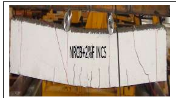
Figure 12 RC beam reduced shear reinforcement with 20kg/m³
