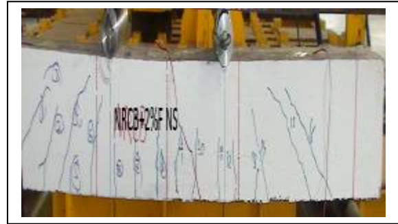
Figure 10 RC beam full shear reinforcement with 20kg/m³
